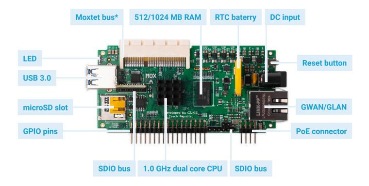
MOX A is available in two variants – 512 MB RAM and 1024 MB RAM. The first one is included in the MOX Pocket Wi-Fi, Power Wi-Fi and Classic, the second one in the MOX Start, which is the starting point for a customized network solution composed of Turris MOX components. The MOX A module is supplied only as a part of the MOX sets, including power supply, microSD card and plastic chassis. It is sold separately only after previous arrangement and only in larger quantities.
